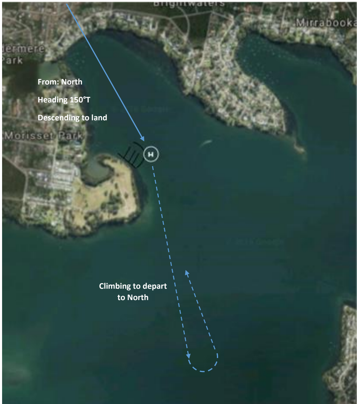
Alternate Approach Path C for South West, South, South East winds. This is an Alternate to Path B2.
