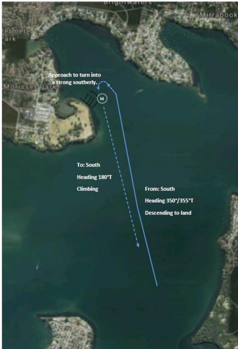
Approach Path B2 designed to meet South East, South, South West winds.
