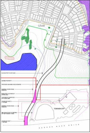
Figure 1 - Detail of southeastern portion of the original Concept Application plan showing the location of the new southern access road to George Bass Drive
