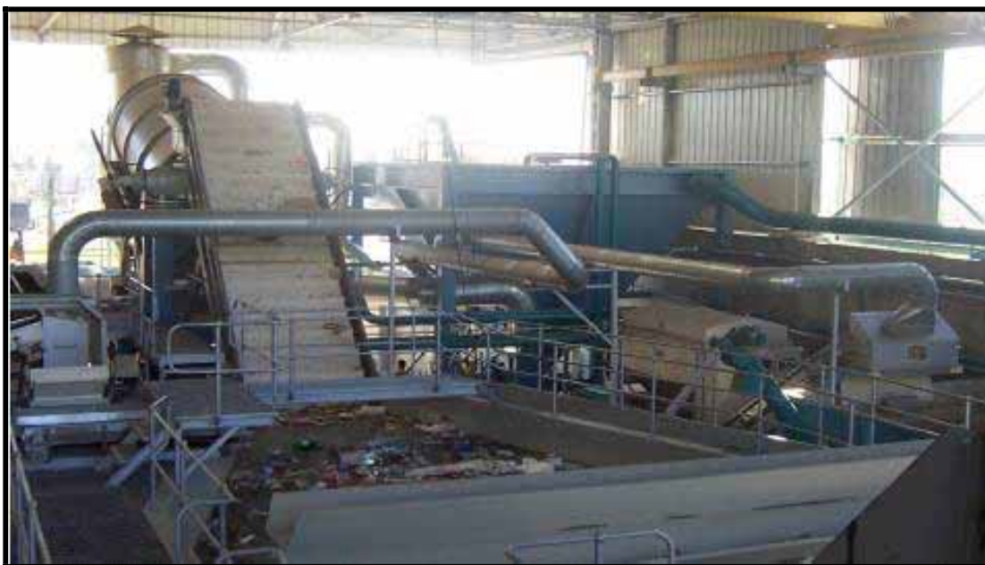
Figure 3.6: Hydro-Mechanical Sorting Systems in the Receiving Hall at Tel Aviv
