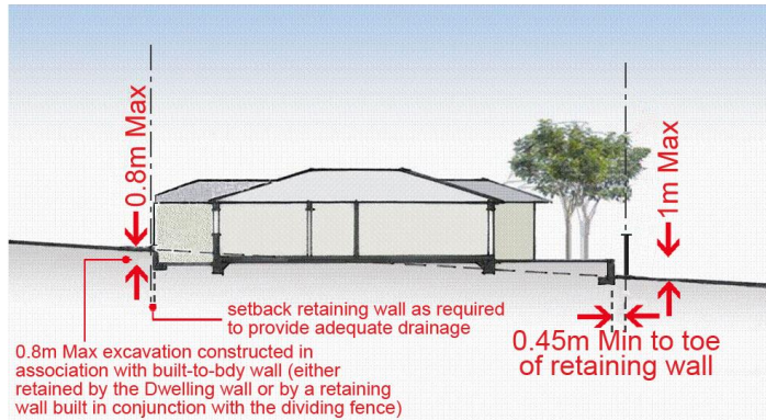
Figure 3.1.1.1 Retaining walls and unprotected embankments
