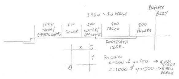
The above sketch indicates that a 4m wide verge could generally accommodate the proposed system with a 750mm vertical clearance. The required verge width would need to increase to 4.5m if the 750mm vertical clearance between water and sewer cannot be achieved, or if the third pipe is inserted on the same side.
