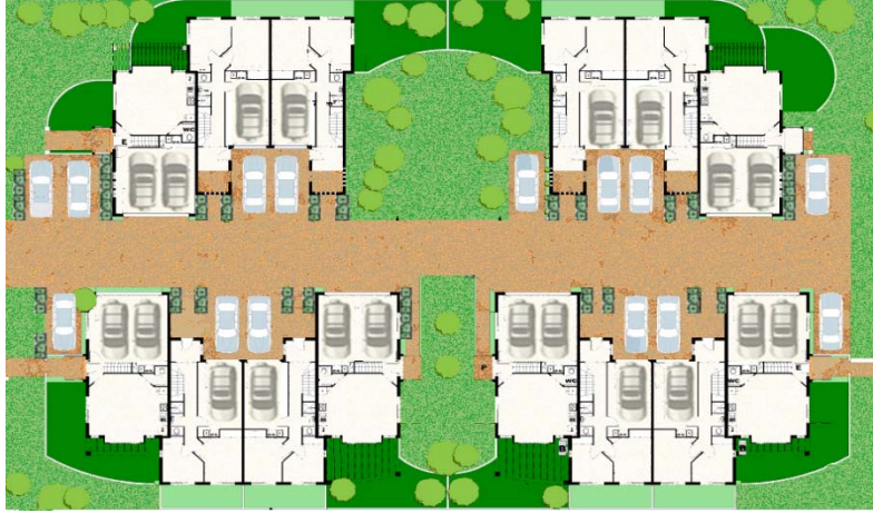
Figure 3.3.1.1 Multi Dwelling Housing illustrating one site with separate titles sharing a common driveway which might be created by either reciprocal easements or common property
