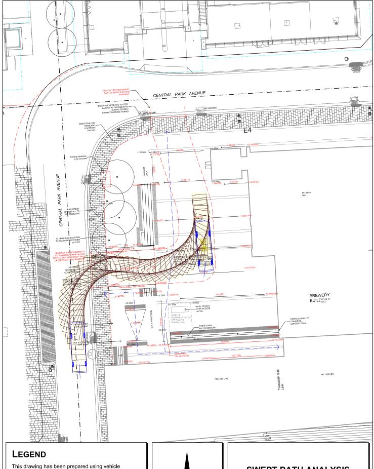
This drawing has been prepared using vehicle modelling computer software AutoTrack V5.00a in conjunction with AutoCAD 2000. The vehicle used is based upon vehicle data provided by Austroads and incorporates a reasonable degree of tolerance. However, it is not possible to account for all vehicle types/characteristics and/or driver ability.
