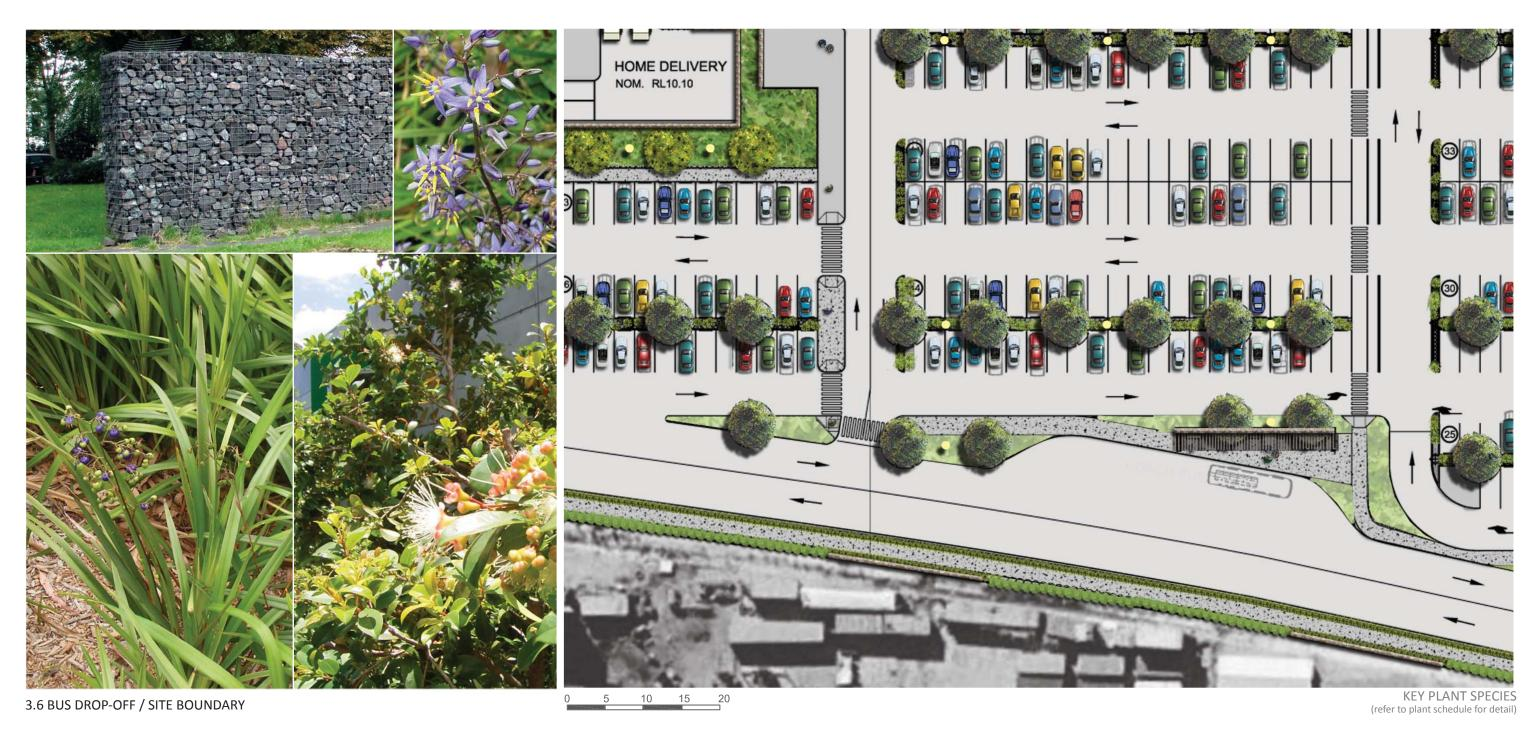
The boundary treatment to the Ikea site, considers the site vocabulary of the Gabion wall while forming a practical barrier and visual buffer to the undesirable view beyond. In this zone, the design is constrained by the overhead flight path being an average of 7m from ground level.
