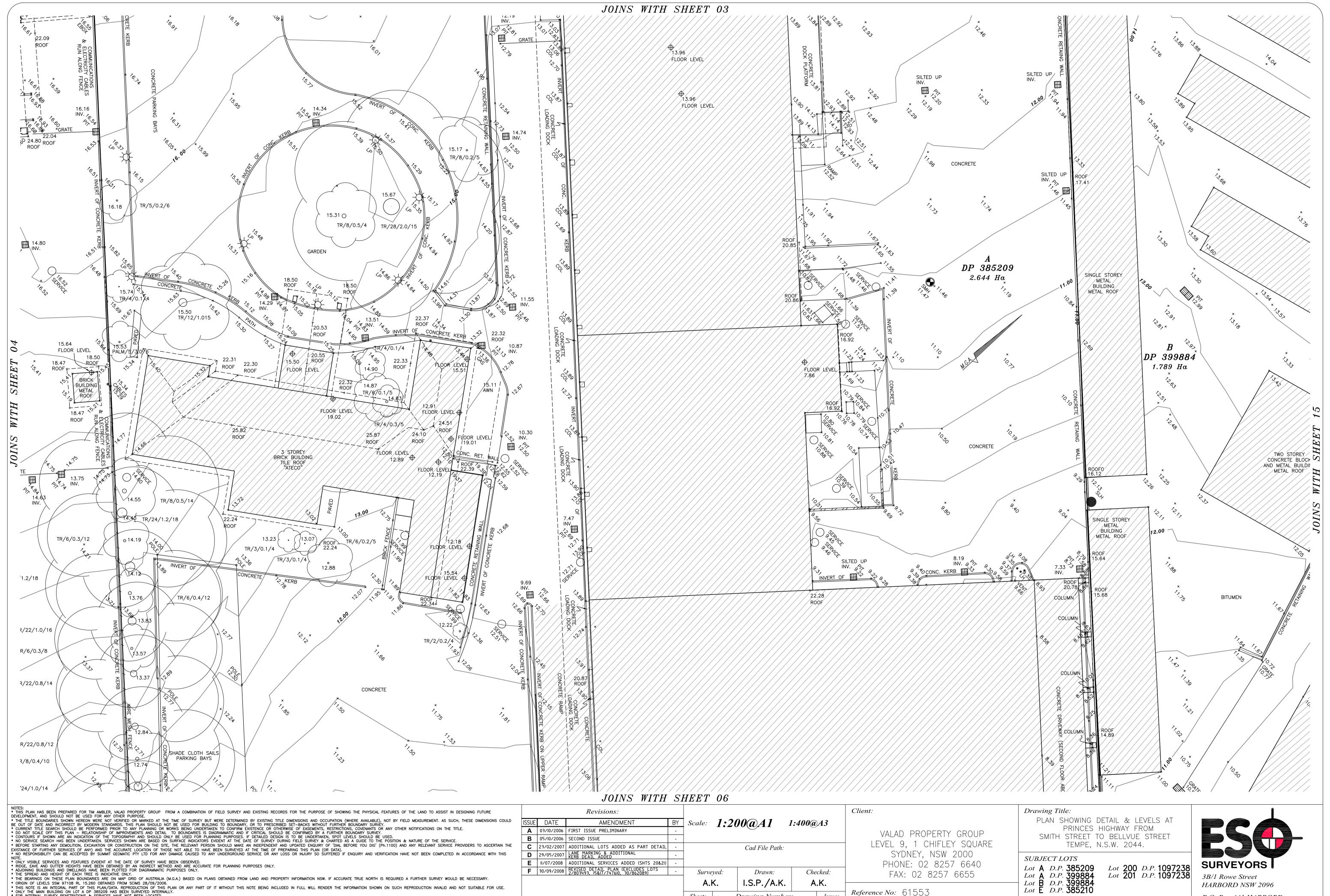
\* THE BEARINGS ON THESE PLAN BOUNDARIES ARE ON MAP GRID OF AUSTRALIA (M.G.A.) BASED ON PLANS OBTAINED FROM EARD AND PROPERTY INFORMATION NSW. IF ACCURATE TRUE NORTH IS REQUIRED A FURTHER SURVEY WOULD BE NECESSARY.
