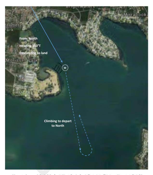
Alternate Approach Path C for South West, South, South East winds. This is an Alternate to Path B2.
