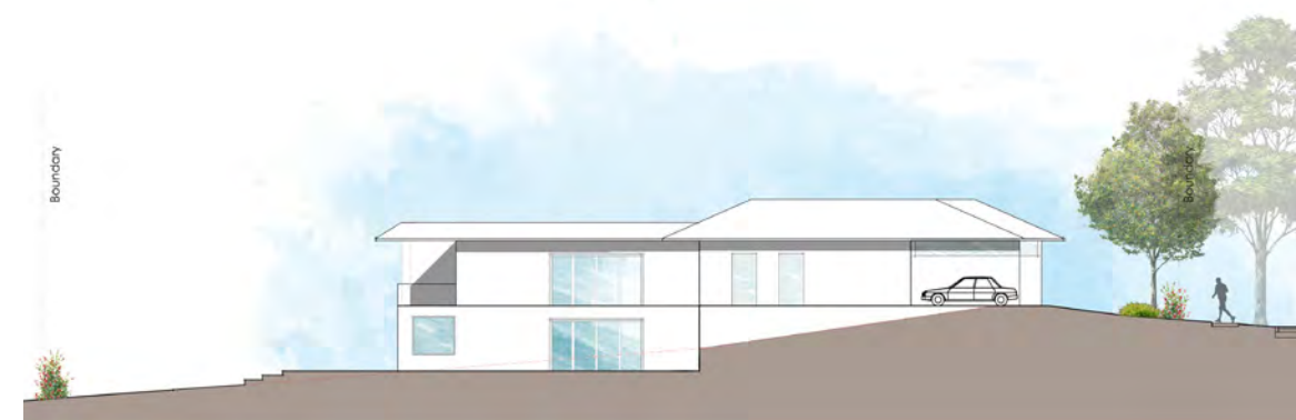
Figure B2.2.8 - Downslope lots side elevation
