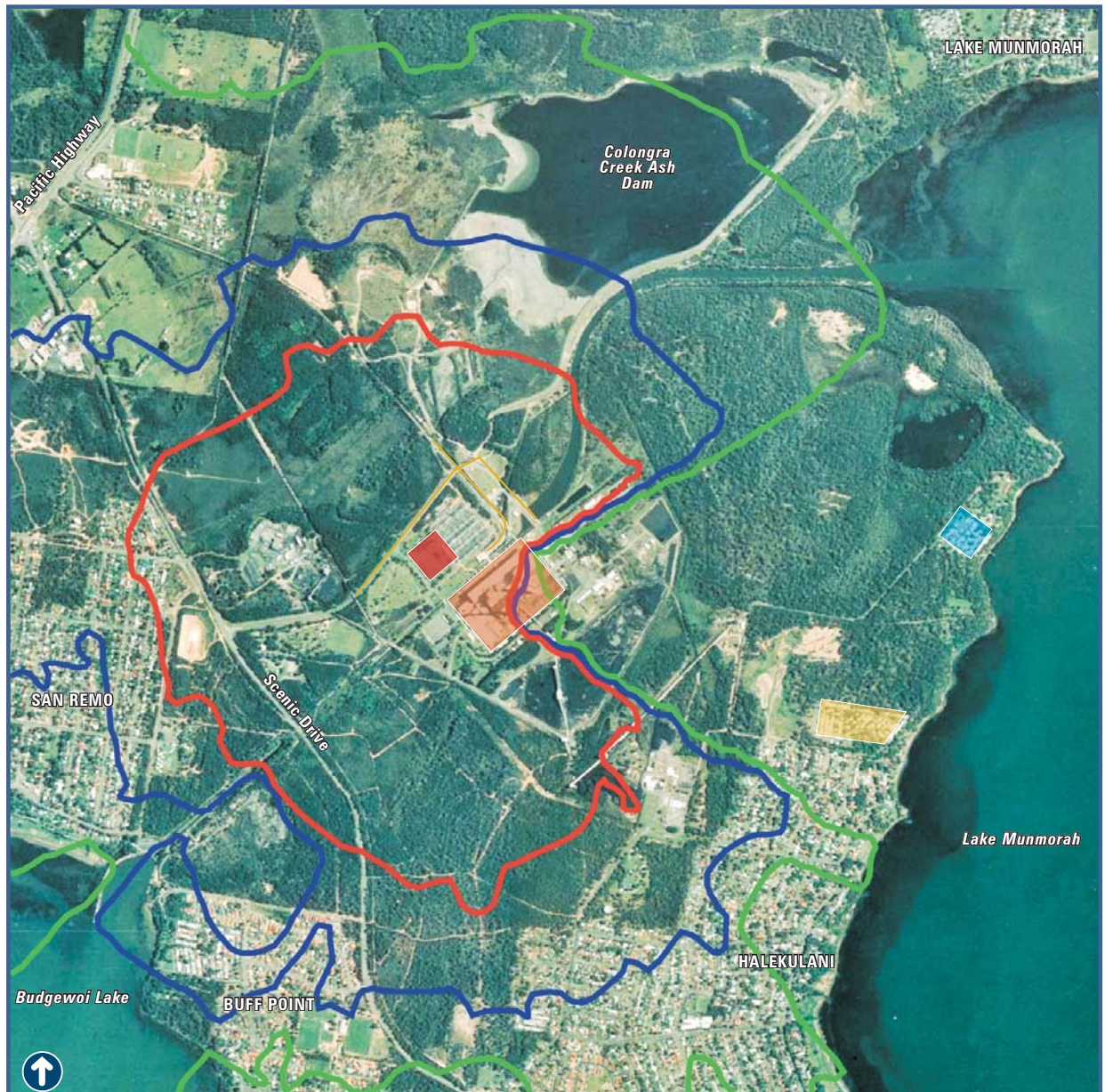
Figure 5.3 Predicted noise level contours (Site A) - Noise enhancing meteorological conditions
