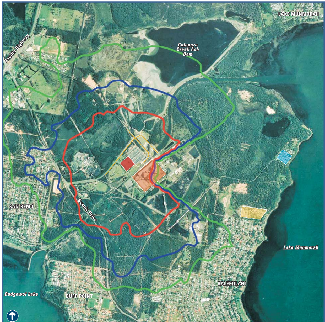
Figure 5.2 Predicted noise level contours (Site A) - Typical meteorological conditions
