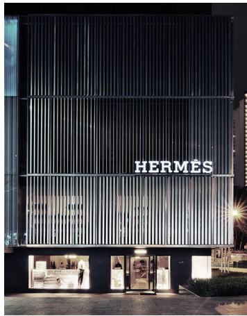
Argyle/Church St corner facade ref image. Metal blades screening in front of existing glazed facade. This allows views out from existing tenancies.
