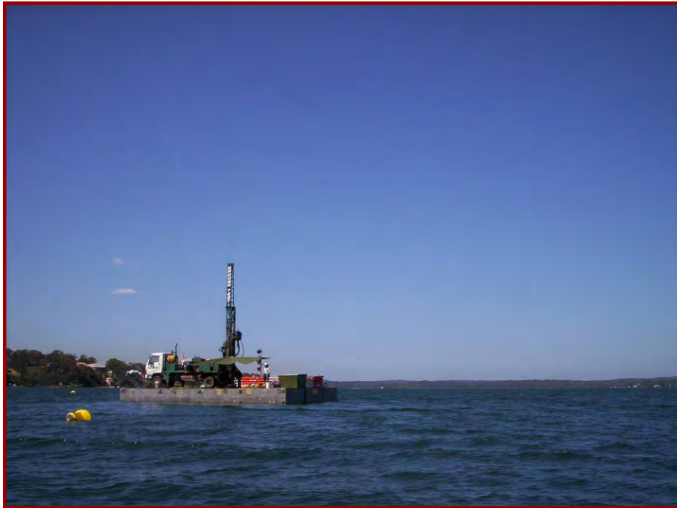
Photo 2 – drill rig set up on modular barge, in proposed marina area
