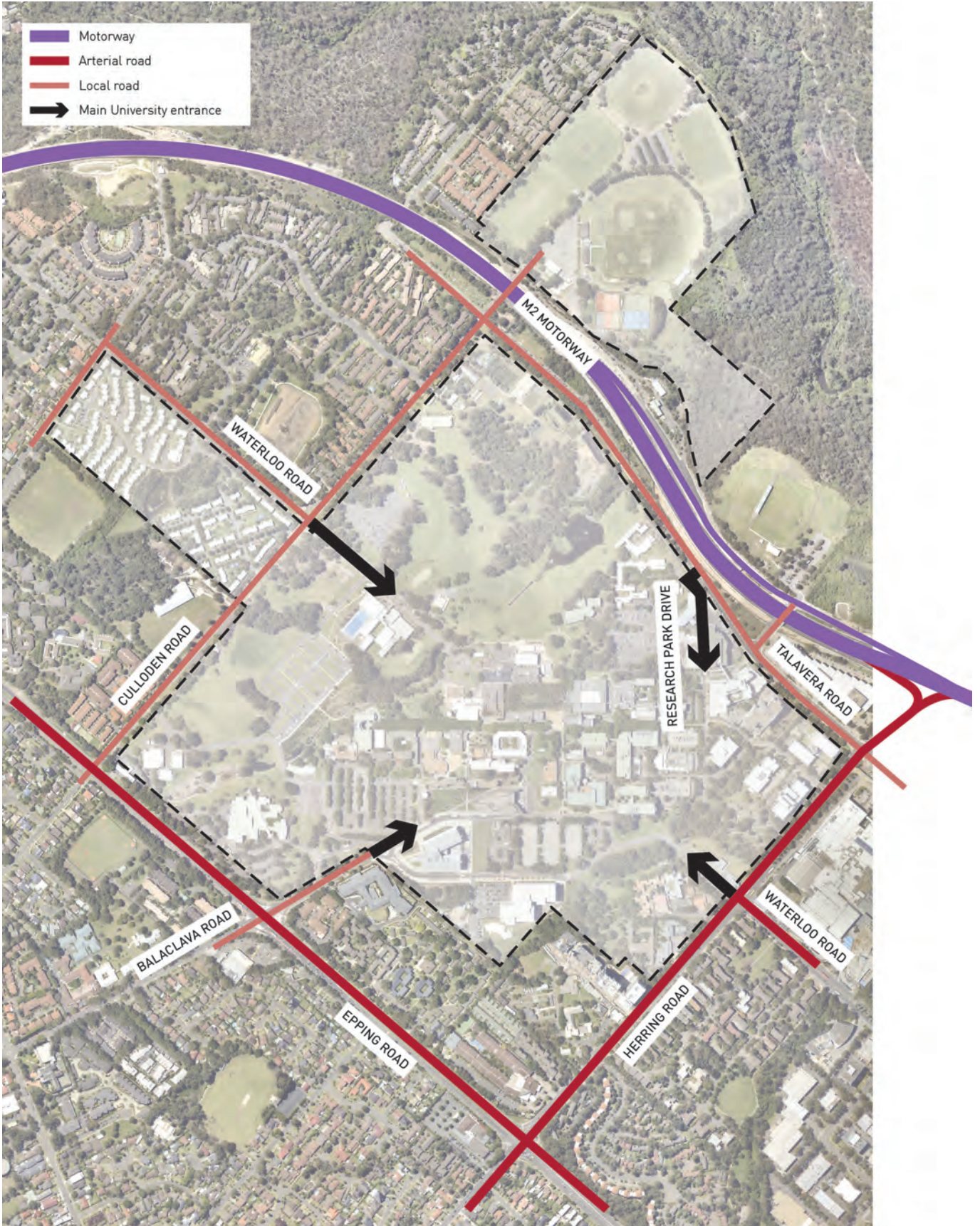
FIGURE 10: EXISTING ROAD NETWORK AND SITE ACCESS
