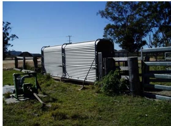
**Plate 2:** Spray race structure and PTO driven pressure pump.
