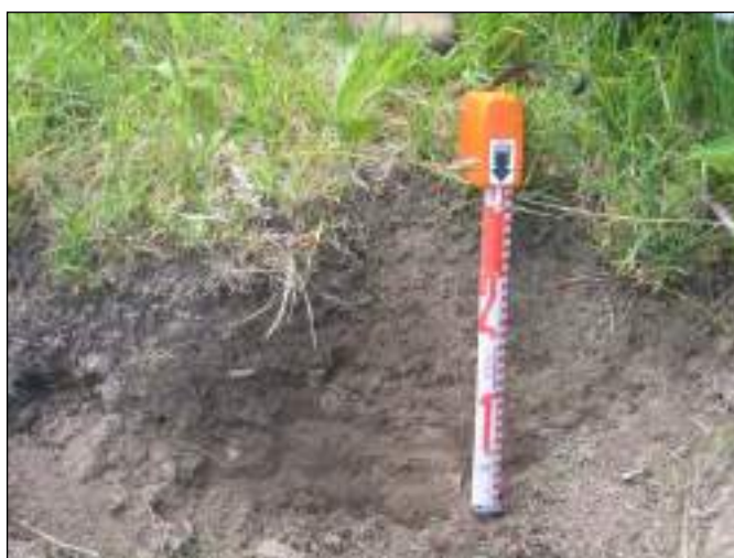
Figure 12. Exposed soil in trailbike “jump” showing retention of topsoil. [MDCA 2005]
