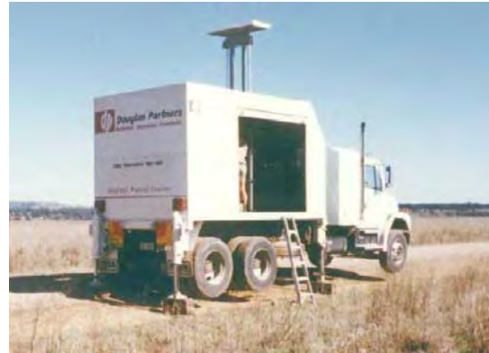
Figure 2: Purpose built CPT rig
