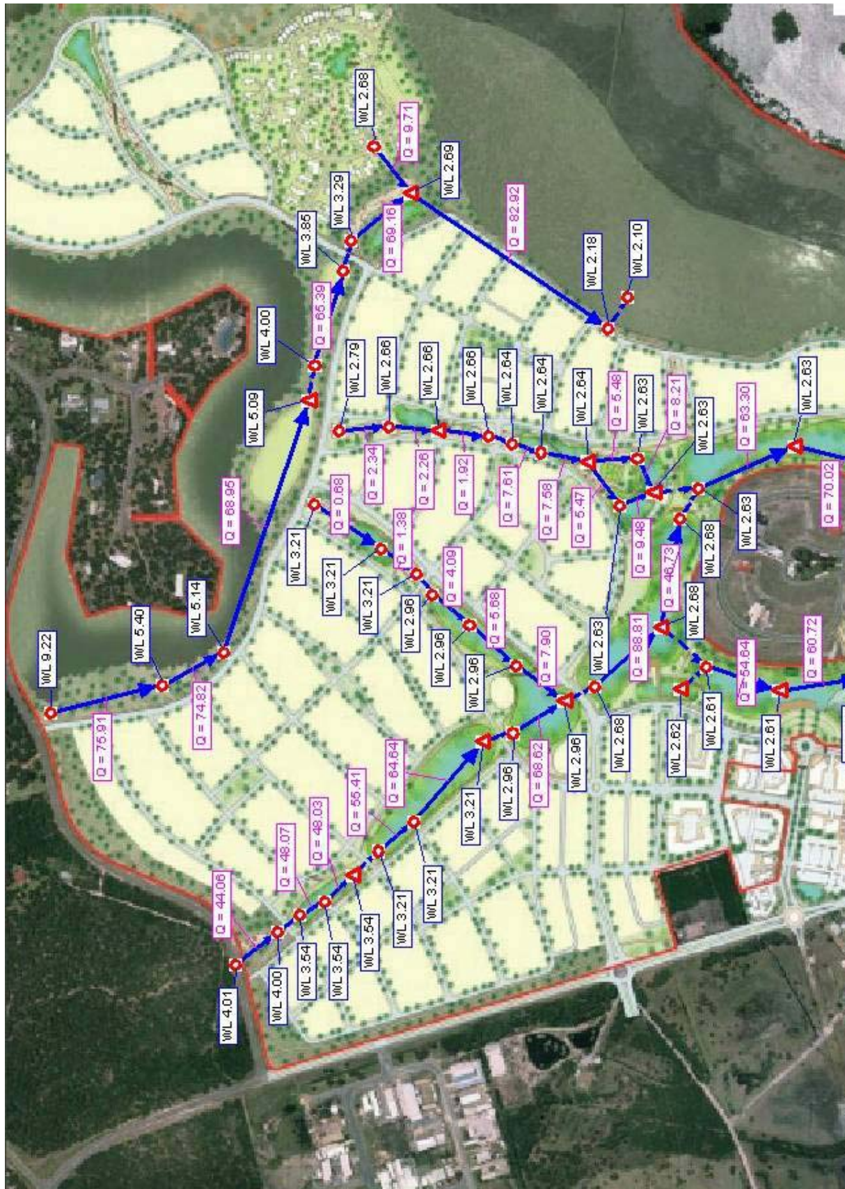
Figure 6 PMF Levels under a 1 Hour PMP Storm
