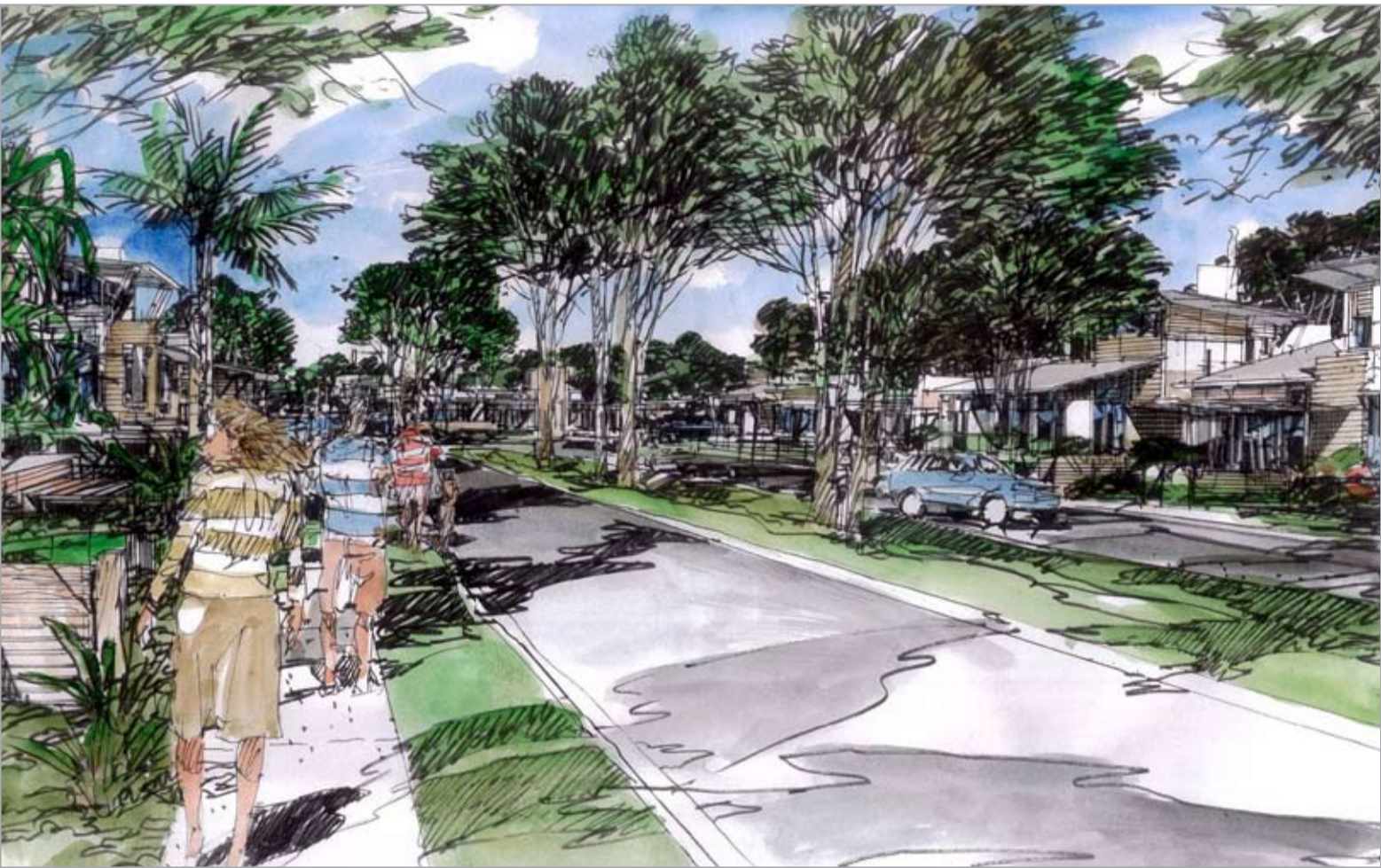
Early concept design for the central greenway of the Eastern Neighbourhood The design has been refined to provide a wider median with drainage by open swales.
