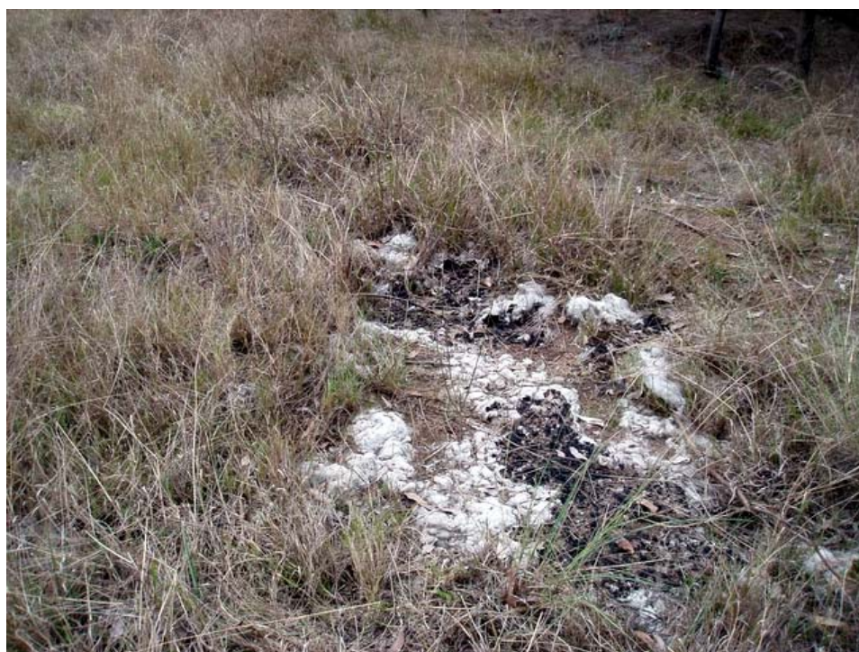
PHOTO 22: Dumped lagging, possible asbestos or other synthetic mineral fibre (SMF), Parcel 2.
