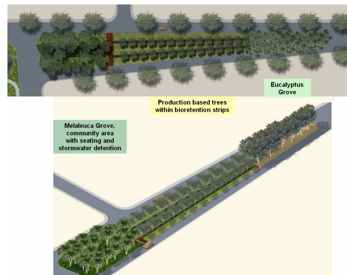
Figure 5-2 Eco-median zones; incorporate water quality and detention functional elements (EDAW)
