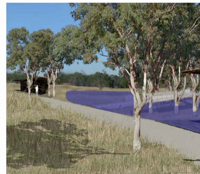
Figure 5–14 Shallow inundation of floodplain areas to manage peak flows from urban development areas.
