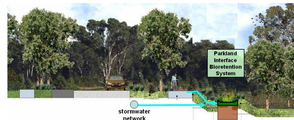
Figure 5-5 Linear bioretention systems on the interface with the parklands.
