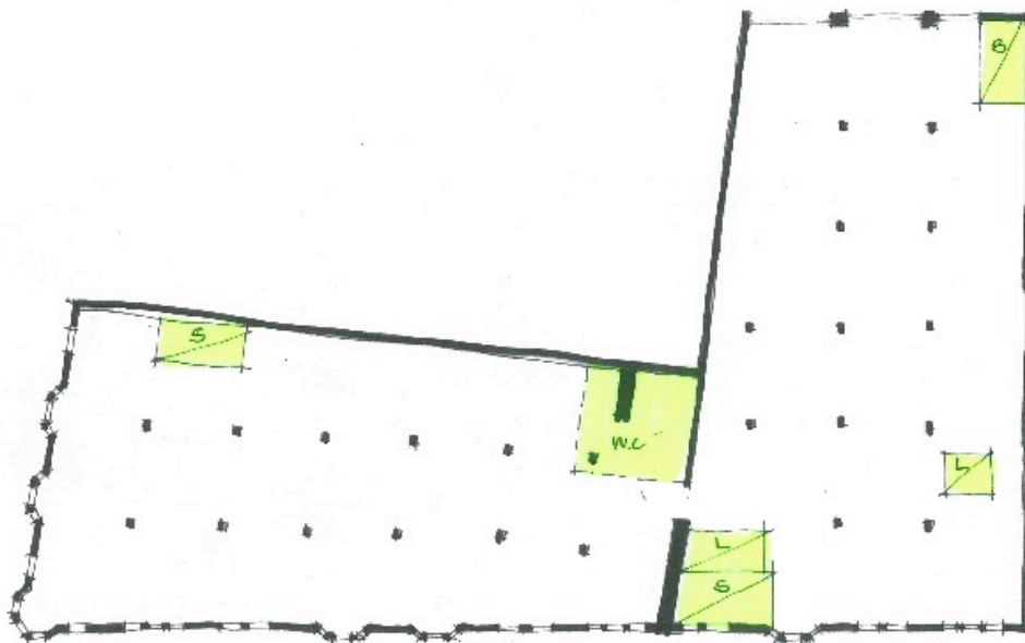
Figure 7: Bon Marche Building Levels 3 and 4. The floor has had relatively little overall change (although now subdivided with new services throughout). The timber column grid and timber floors appear to remain on much of the floor. The areas shaded yellow have had changed levels, floors removed and new elements such as stairs and lifts inserted.
