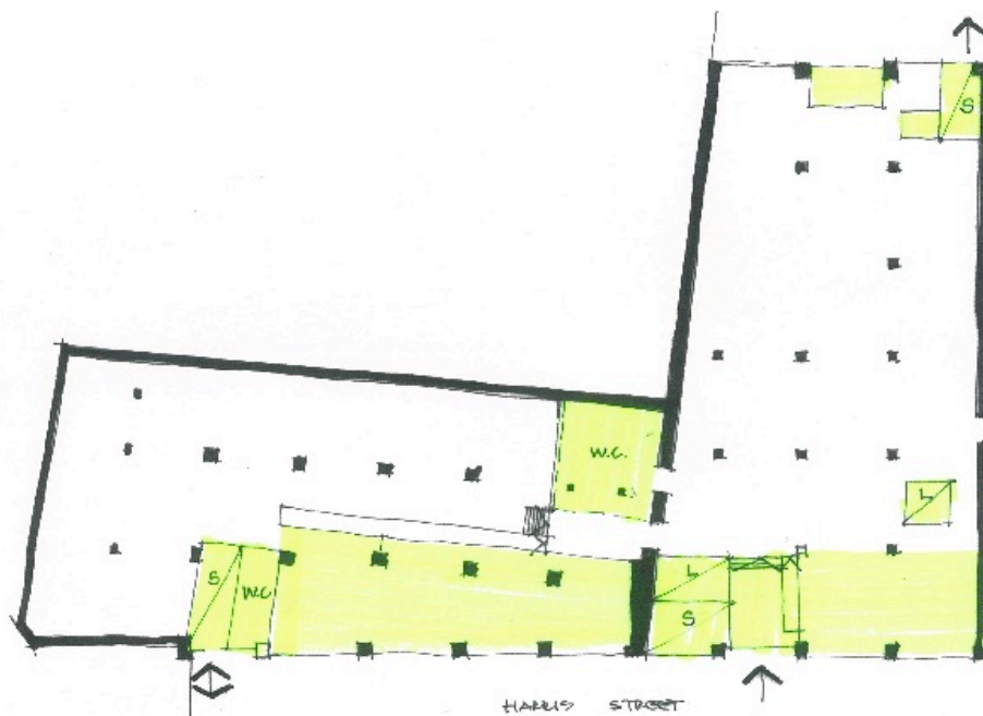
Figure 5: Bon Marche Building Level 1. The left hand end of the building (south) is a basement below Broadway with the shopfronts, added in the 1970s stepping down as Harris Street falls to the north. The former loading docks, occupying the northern 6 bays of the building have been infilled with new floor levels. The areas shaded yellow have had changed levels, floors removed and new elements such as stairs and lifts inserted.
