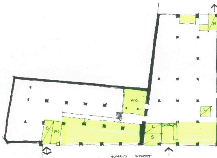
Figure 70: Bon Marche Building Level 1. The left hand end of the building (south) is a basement below Broadway with the shopfronts, added in the 1970s stepping down as Harris Street falls to the north. The former loading docks, occupying the northern 6 bays of the building have been infilled with new floor levels. The areas shaded yellow have had changed levels, floors removed and new elements such as stairs and lifts inserted.
