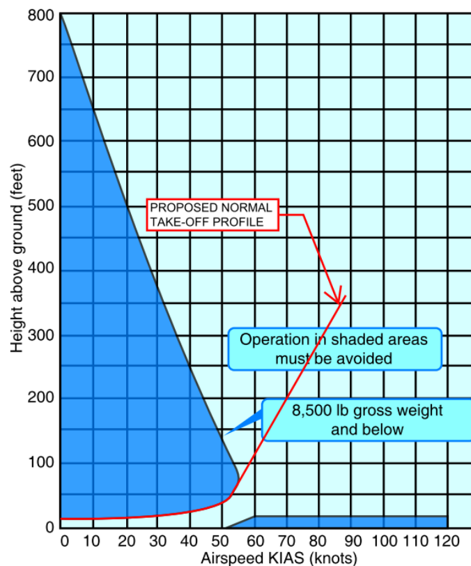
Figure 3.2 Height vs velocity chart for aircraft below 3,856kg (US FAA, Helicopter Flying Handbook, 2012)
