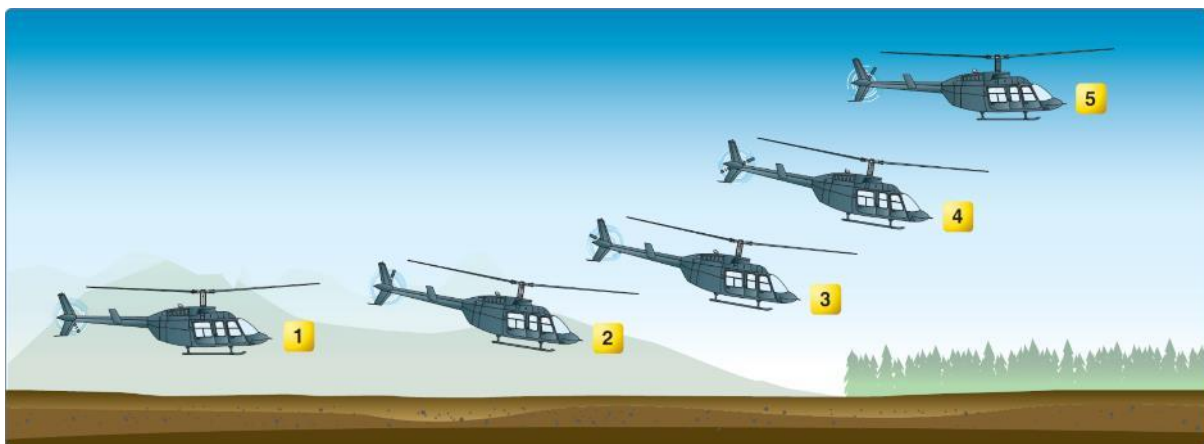
Figure 3.1 Helicopter profile during a normal take-off from hover
