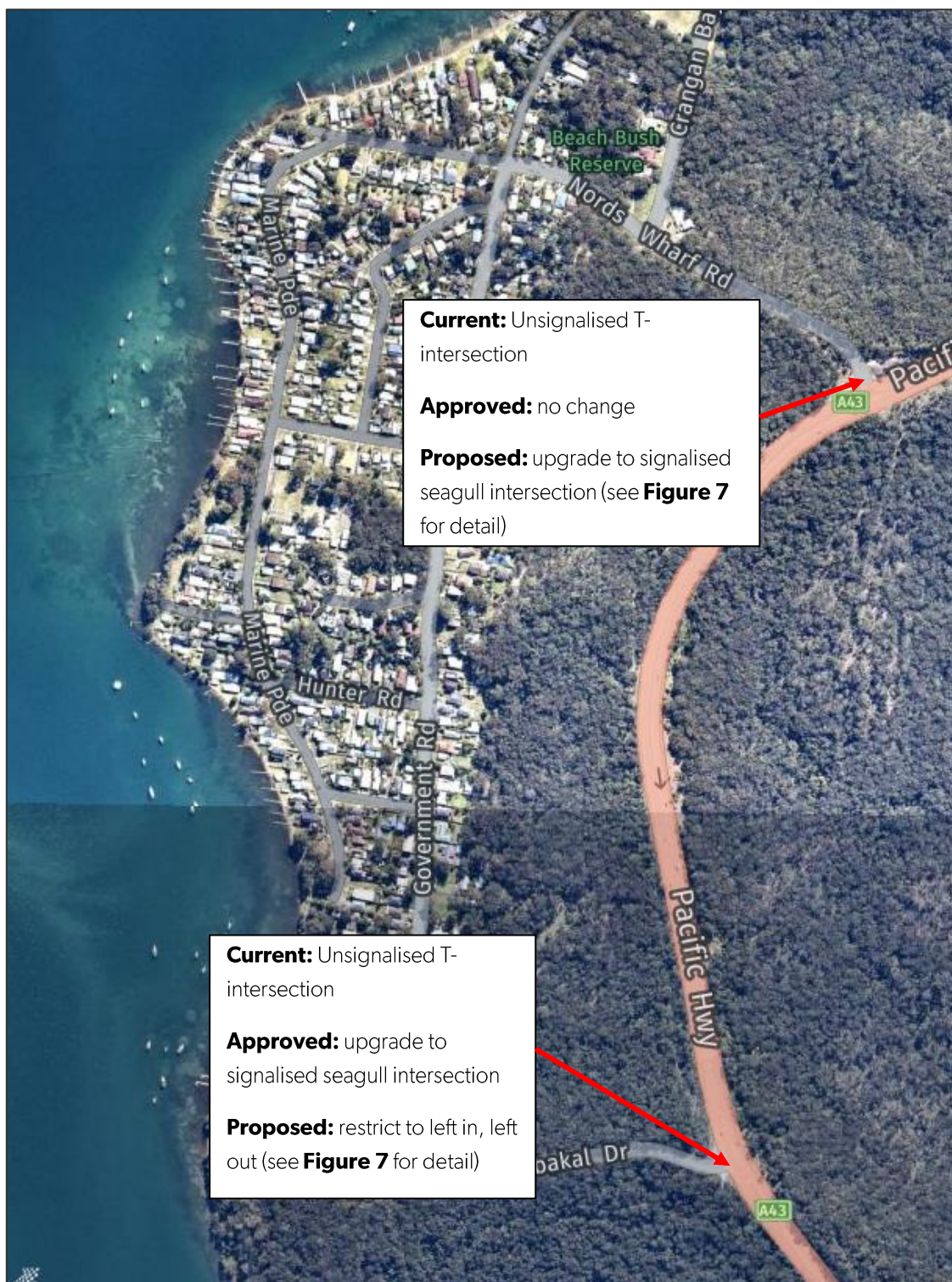
Figure 7 | Approved and proposed intersection treatment
