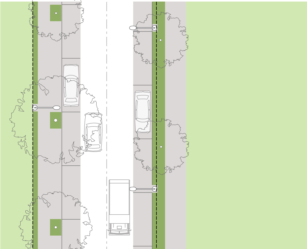
Road type 1B 15m collector road at park (10.9 pavement)
