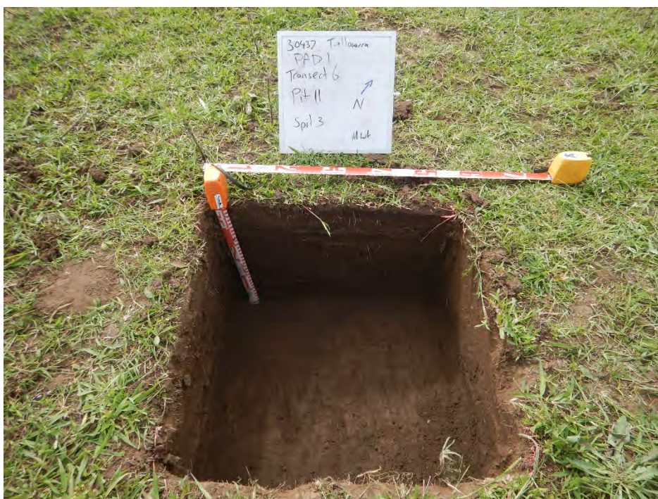
Plate 26 Low potential area, test pit 11, showing soil profiles
