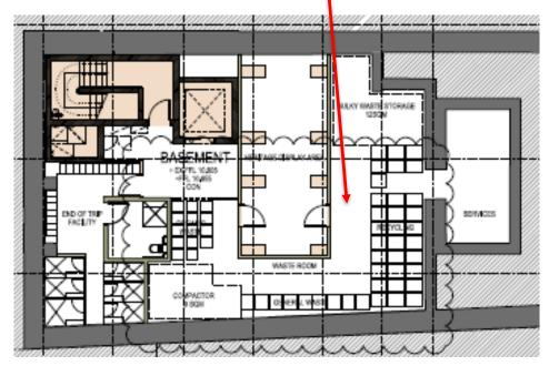
The design of the waste room is approximately  $68.0 \text{ m}^2$ . As indicated above, there is a requirement for bins of  $21.5 \text{ m}^2$ . An allowance of 30% is recommended so this results in a space requirement of  $28.62 \text{ m}^2$ .
