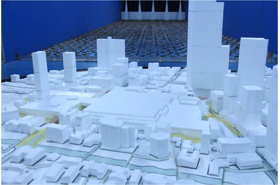
Figure 1k: Photograph of the Wind Tunnel Model – Existing Scenario (close up view from the south-east)
