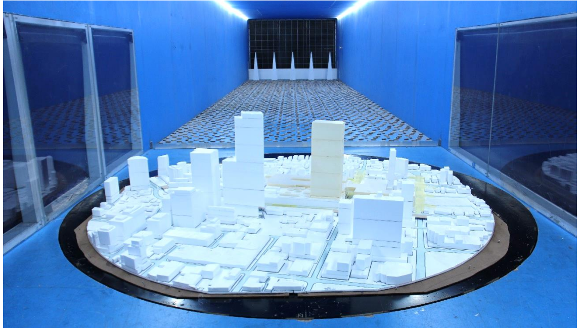
Figure 1a: Photograph of the Wind Tunnel Model – Proposed Scenario (view from the north)
