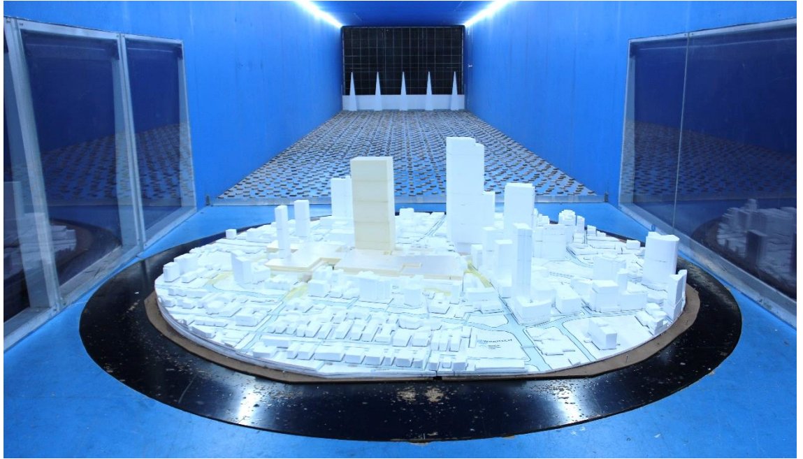
Figure 1c: Photograph of the Wind Tunnel Model – Proposed Scenario (view from the south)
