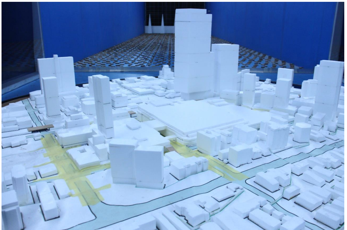
Figure 1l: Photograph of the Wind Tunnel Model – Existing Scenario (close up view from the south-west)
