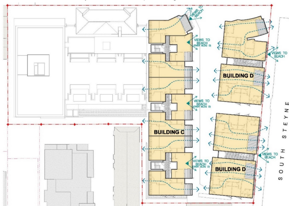
Figure 20: A example reference design floor plan detailing levels of apartment cross ventilation paths through residential apartments on a typical level (Building C).
