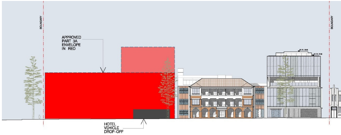
Figure 6: North Elevation with Part 3A massing in red showing limited openness on the ground plane and wide vehicle entry.
