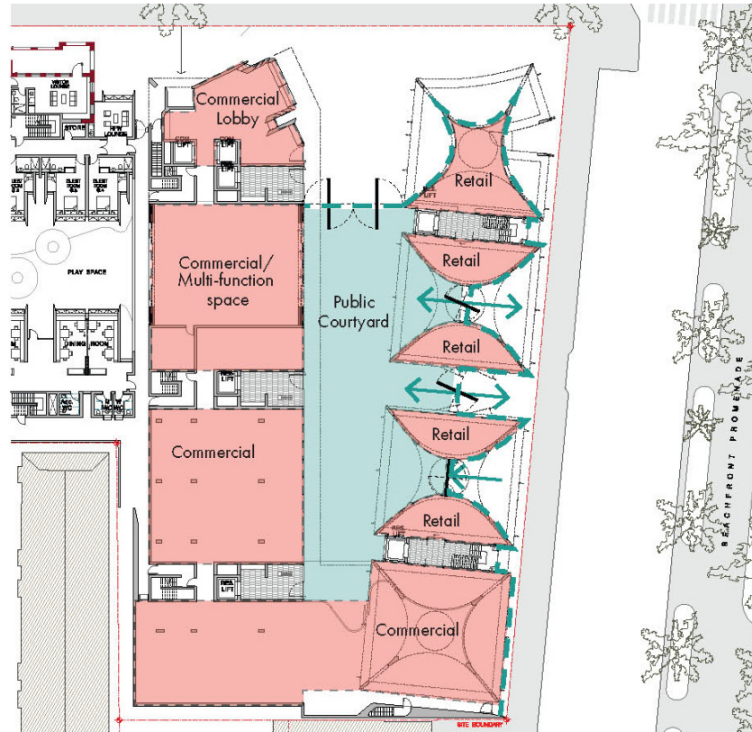
Figure 1: Diagram of proposed perimeter security line (in a dashed green line) for the ground floor level.
