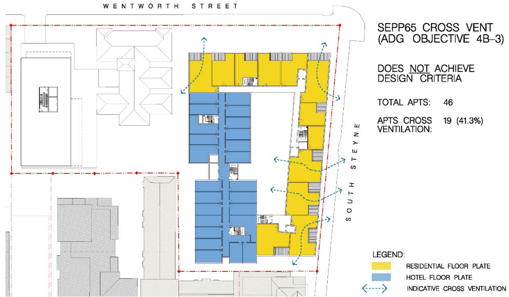
Figure 3: Part 3A Concept Plan - upper-level floor plan diagram examining a possible apartment configuration and the resulting natural ventilation outcomes.
