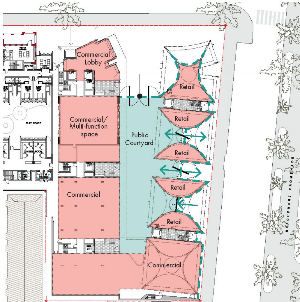
Figure 17: An illustration of the ground floor secure perimeter to the courtyard space.
