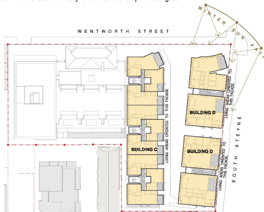
Figure 12: An example reference design floor plan detailing noting residential apartment solar access (Building C).
