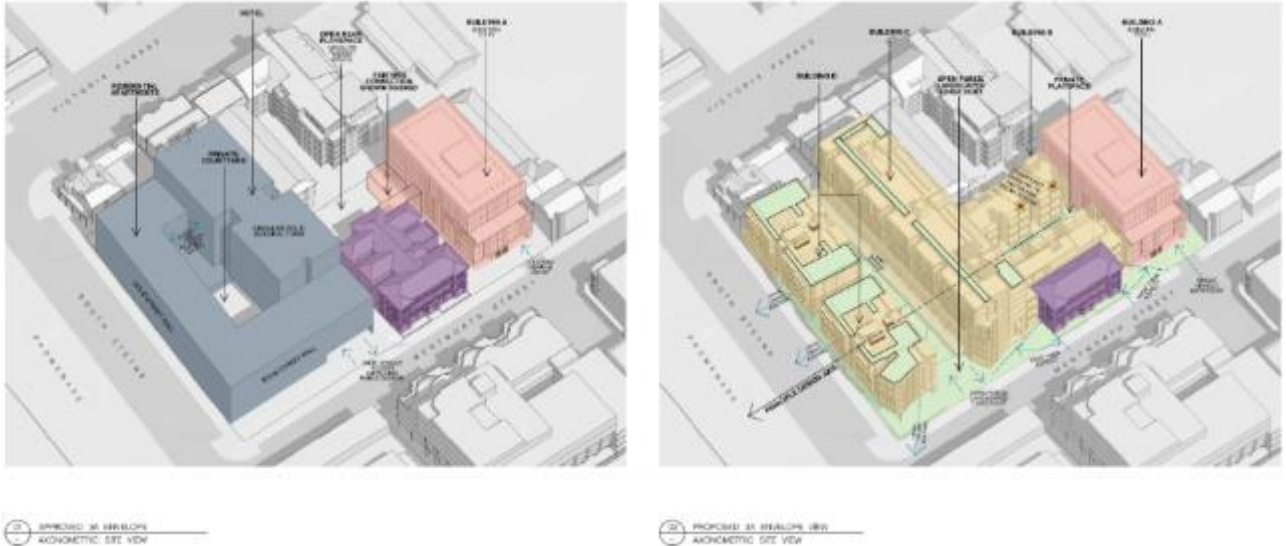
Figure 33 – Building envelope and massing redistribution diagram (plan extract S75W – 1354)
