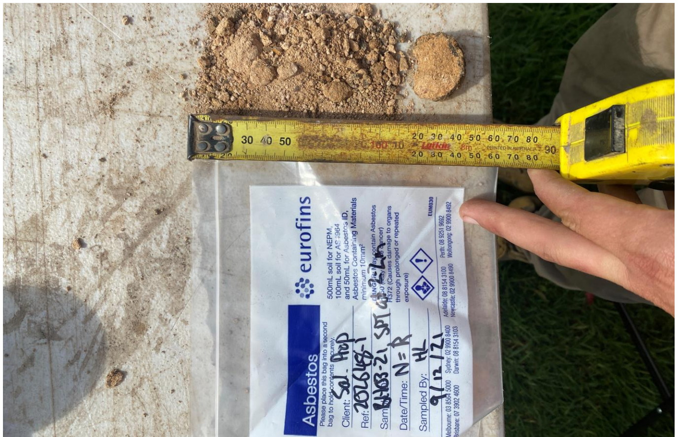
BH03-21, SPT at 2.2m, N=R
