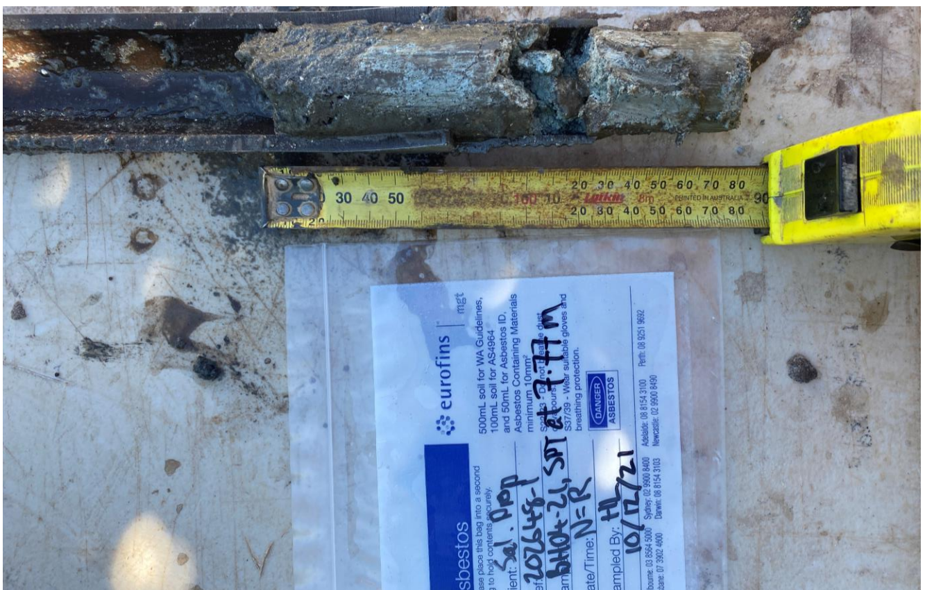
BH04-21, SPT at 7.77m, N=R
