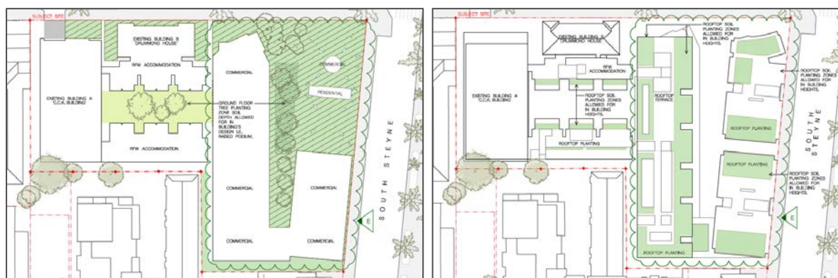
Figure 24 | Plans showing the ground floor tree planting zones (left) and rooftop planting zone (right) (Source: Proponent's Response to Submissions)
