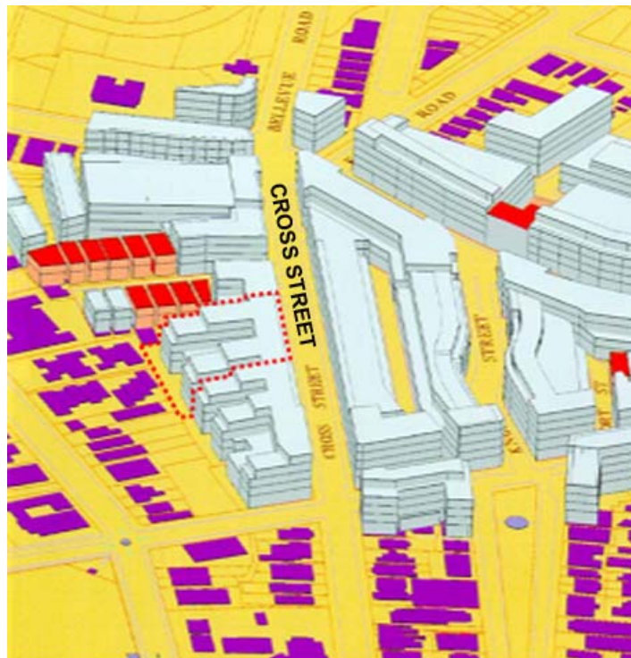
Figure 5. Double Bay DCP 2002 Envelope Control (2D Image) Source: Double Bay DCP (5.12 View 1)
