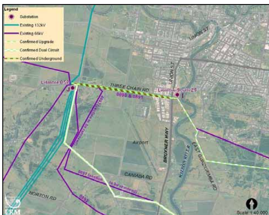
Figure 3.10 Underground Line on Three Chain Road and Dual circuit to Lismore BSP Substation from South
