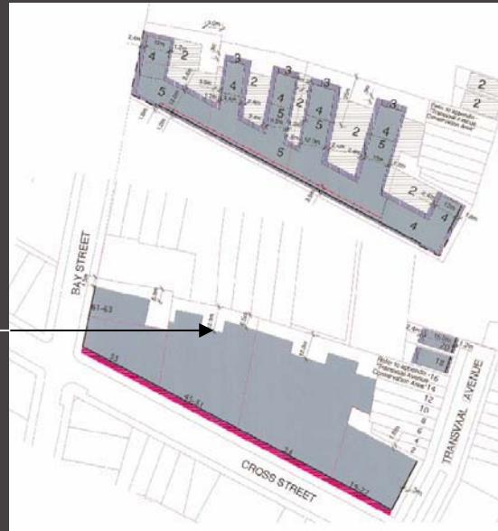
DCP envelope controls
