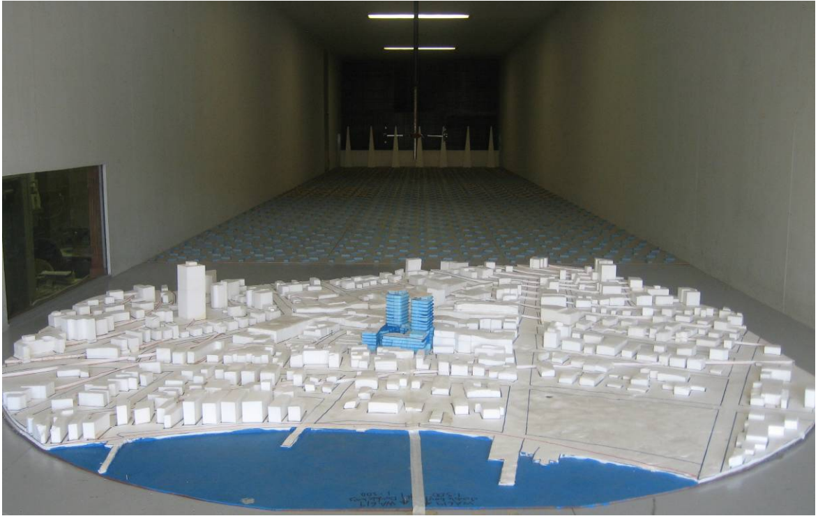
Figure 1d: Photograph of the Model in the Wind Tunnel (proposed development model, view from the North)
