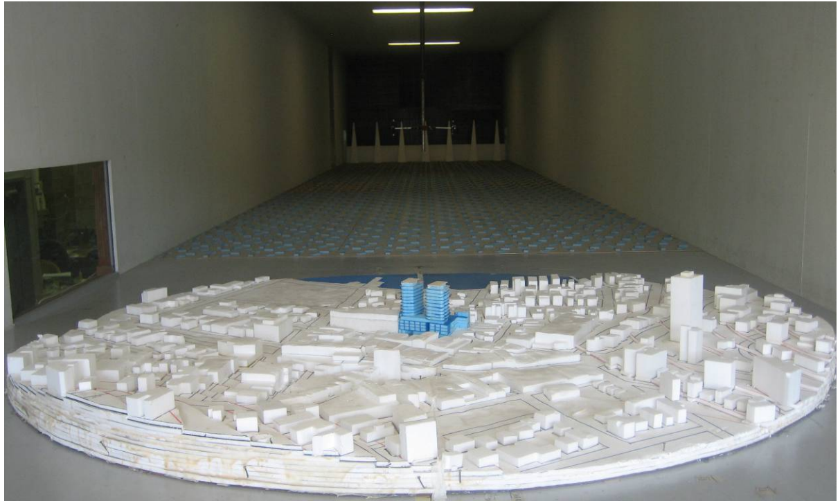
Figure 1b: Photograph of the Wind Tunnel Model (proposed development model, view from the South)
