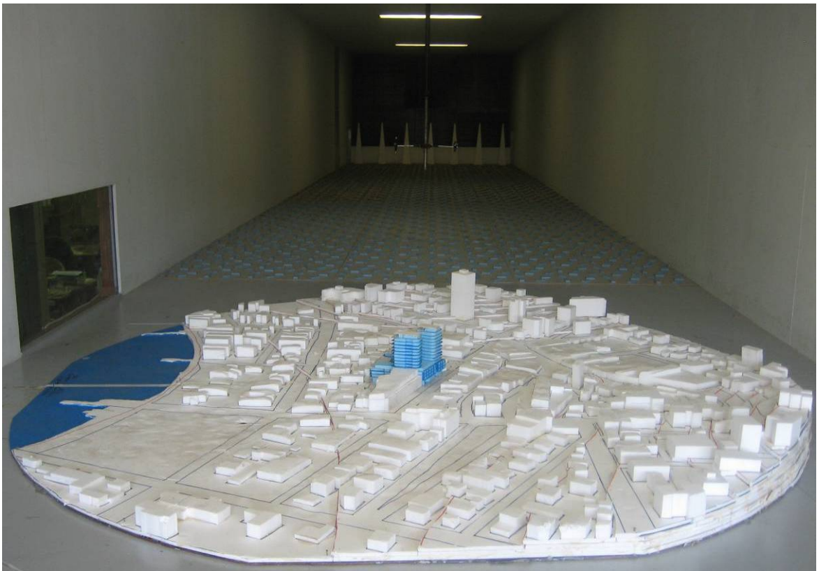
Figure 1e: Photograph of the Model in the Wind Tunnel (proposed development model, view from the West)
