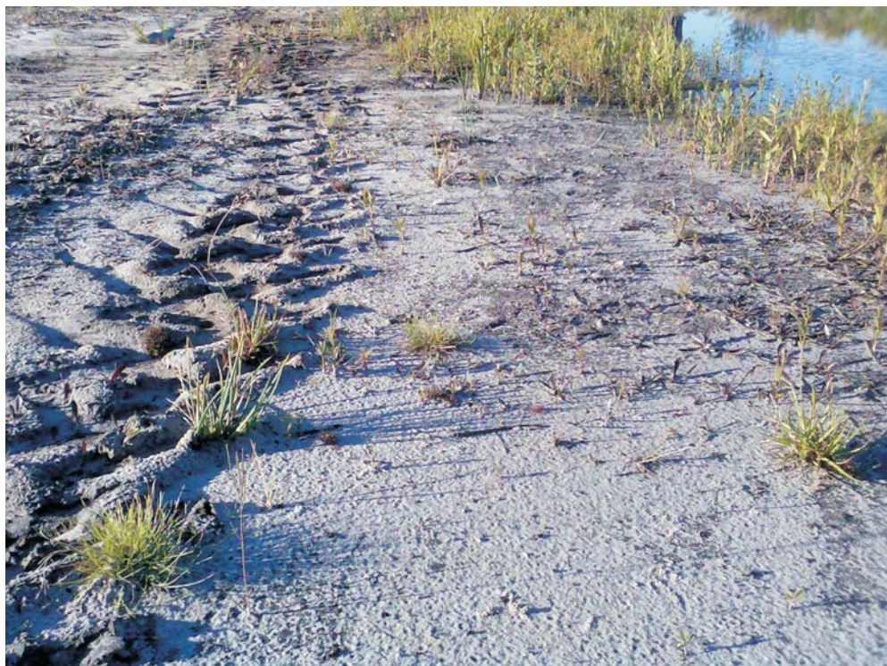
Photo 4: Photographs of the soils in undisturbed and disturbed areas of the site demonstrating the sandy nature of these soils.
