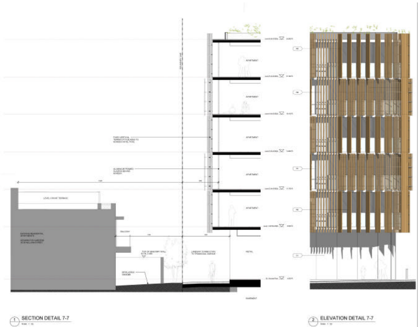
Figure 31. Section through northern podium
