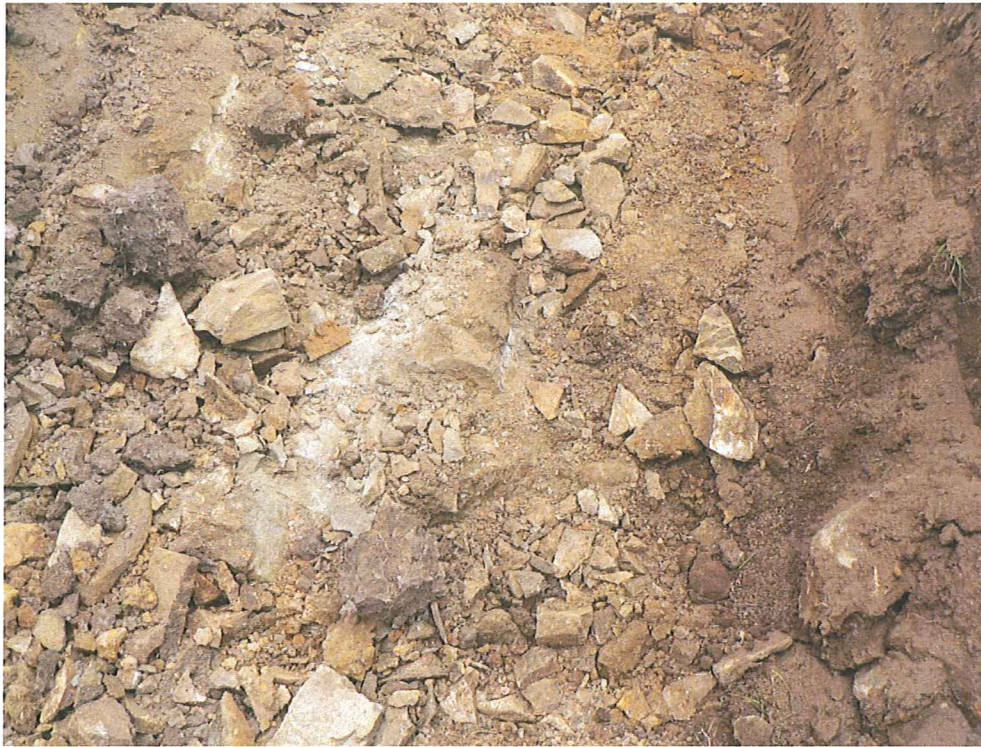
Plate T2A. Chn.6.5m. Refusal on slightly weathered tuffaceous sandstone.
