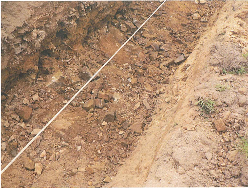
Plate T1A. Chn.4.5m to 10m. Refusal/difficult digging on moderately weathered/slightly weathered tuffaceous sandstone.
