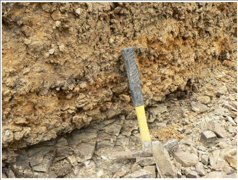
T2C – Gravelly silty clay overlying meta-shale
