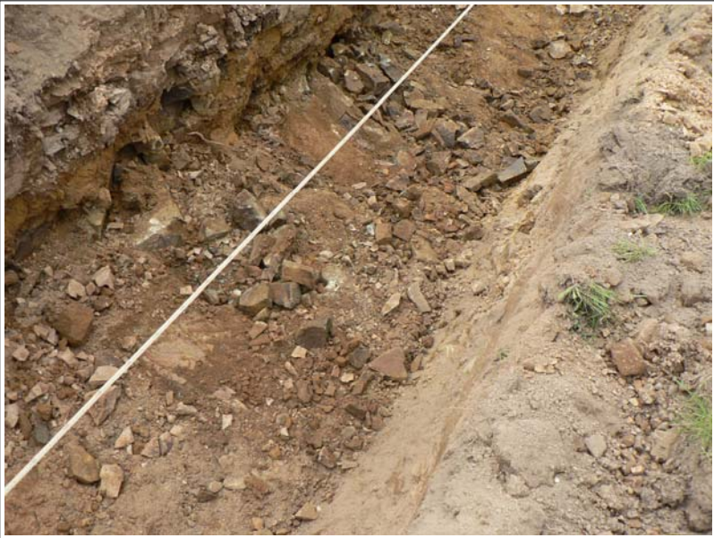
T1A – Refusa/difficult digging on moderately weathered/slightly weathered tuffaceous sandstone
