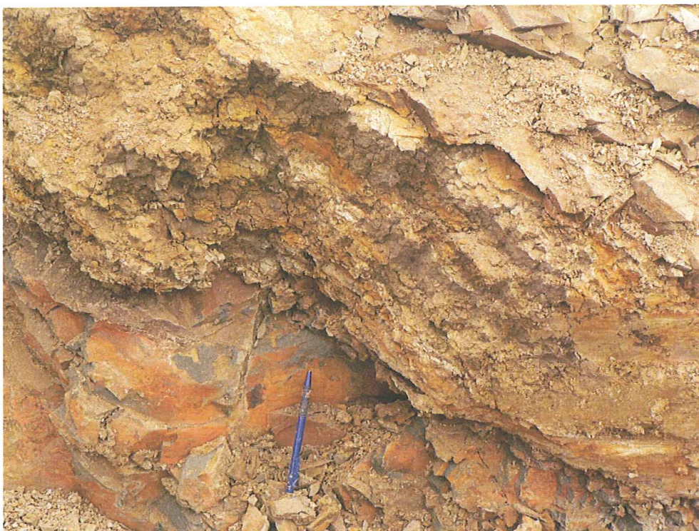
Plate TF5. Chn.11.4m. Fault plane dipping downstream (to the right of the photograph). Brecciated zone overlying meta-shale.
