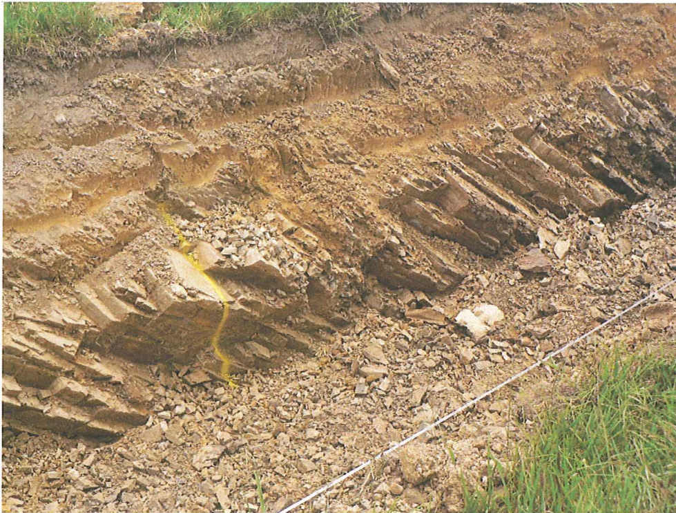
Plate TF13. Chn.37m. Well defined bedding dipping downstream at 40^\circ in direction 073^\circ\text{M} .
