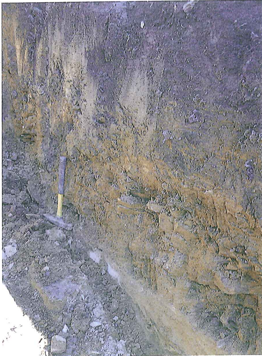
Test Pit TP147. Crushed sandstone layer, 1.05m to 1.20m depth.
