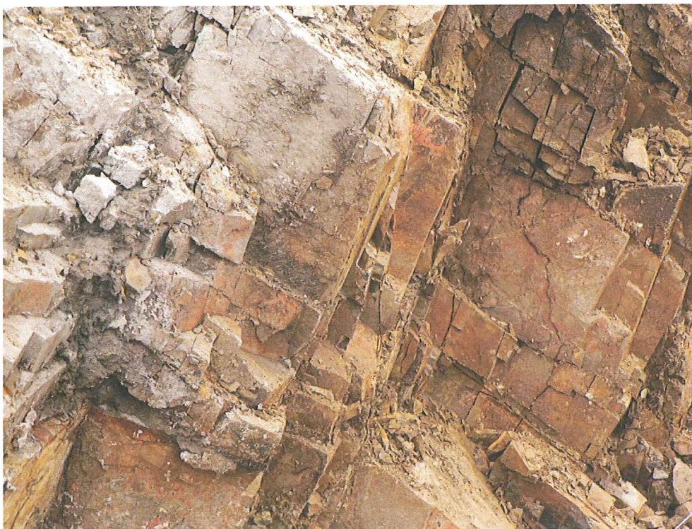
Plate TF2. Chn.8.3m. Meta-shale, dipping upstream at 65° to 70° in direction 275°M.
