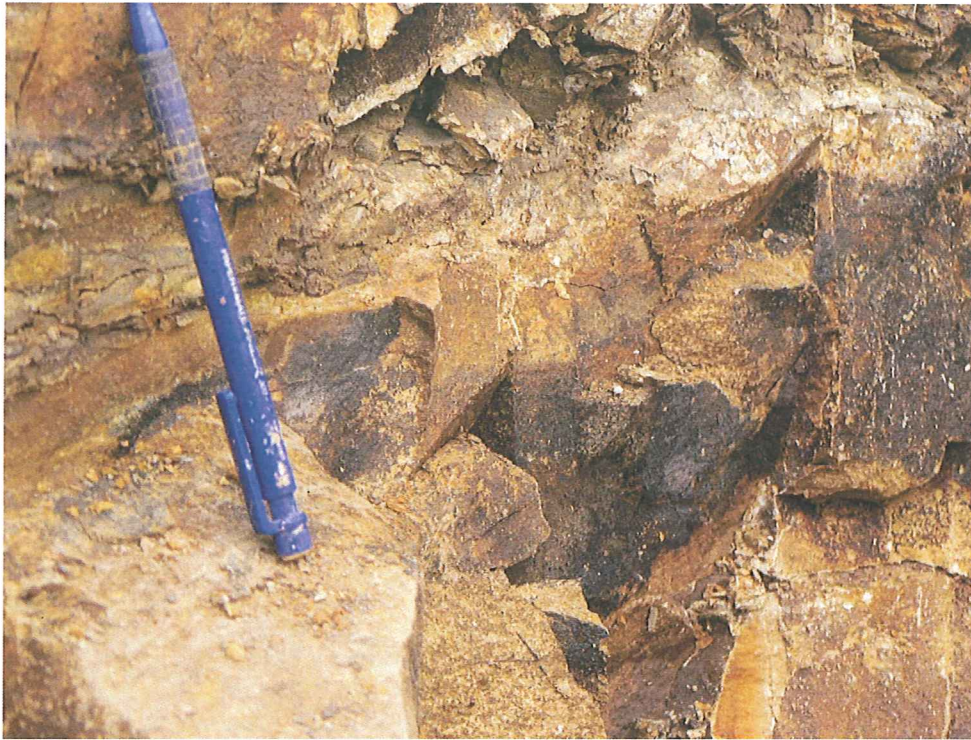
Plate T1C. Chn.9m. Contact between meta-shale and underlying tuffaceous sandstone.
