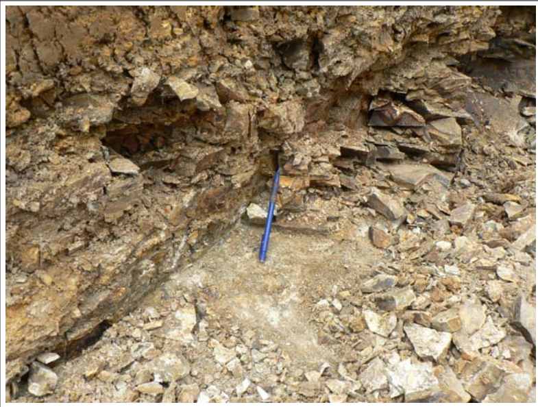
T2B – Contact between meta-shale and underlying tuffaceous sandstone
