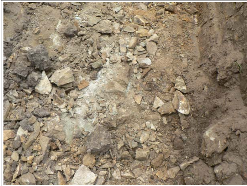
T2A – Refusal on slightly weathered tuffaceous sandstone
