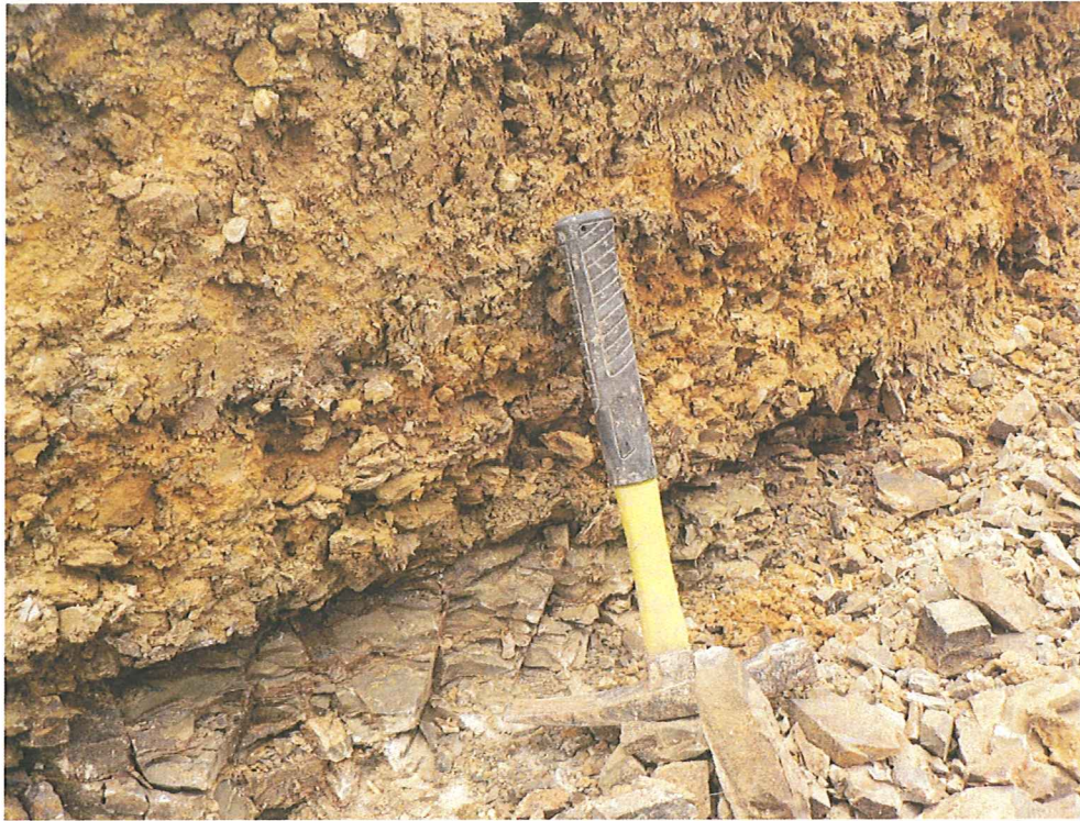
Plate T2C. Chn.10.7m. Gravelly silty clay overlying meta-shale.
