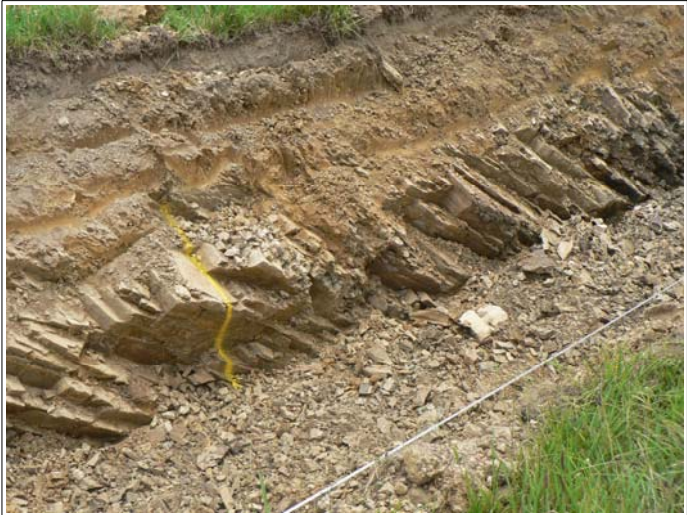
TF13 – Meta-shale, bedding dipping downstream at 40°
