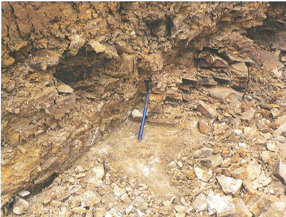
Plate T2B. Chn.9.5m. Contact between meta-shale and underlying tuffaceous sandstone.
