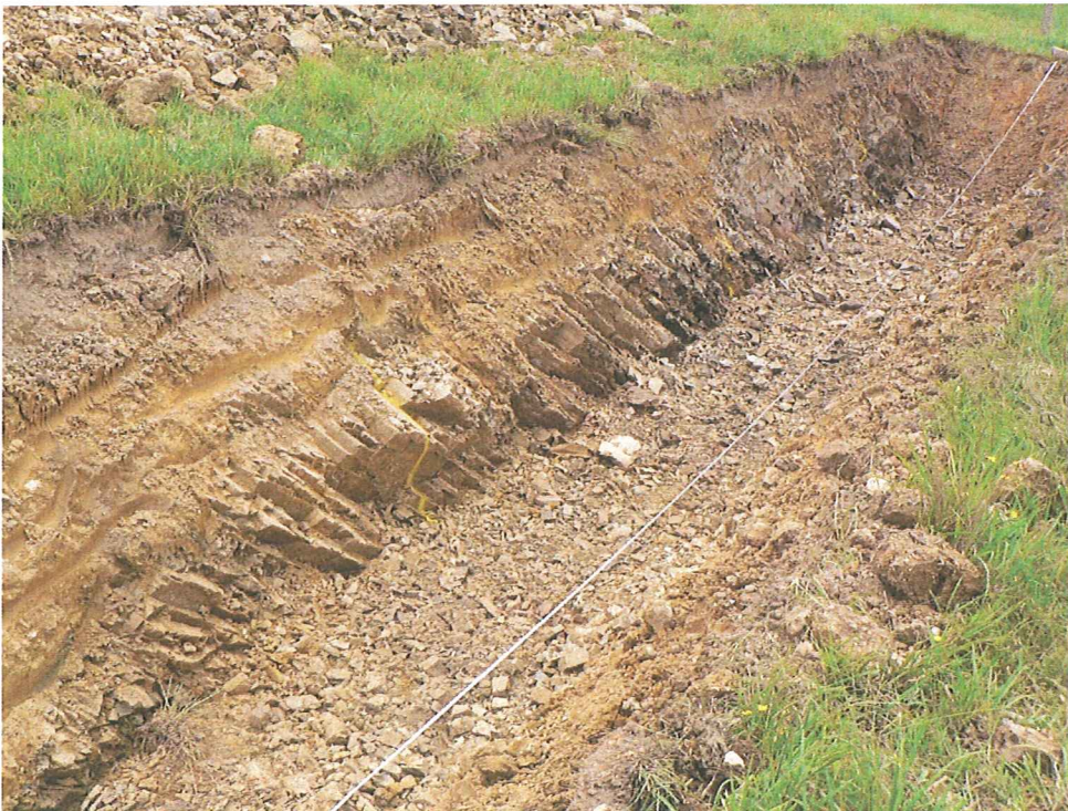
Plate TF12. Chn.37m to 52m. General view of the meta-shale downstream of the fault zone (dipping downstream at 40^{\circ} to 30^{\circ} in direction 060^{\circ}\text{M} to 072^{\circ}\text{M} ).
