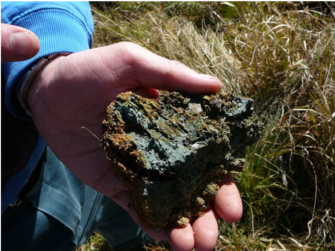
Photo 12: TP142 Lower slide plane, thin clay seam in extremely weathered rock
