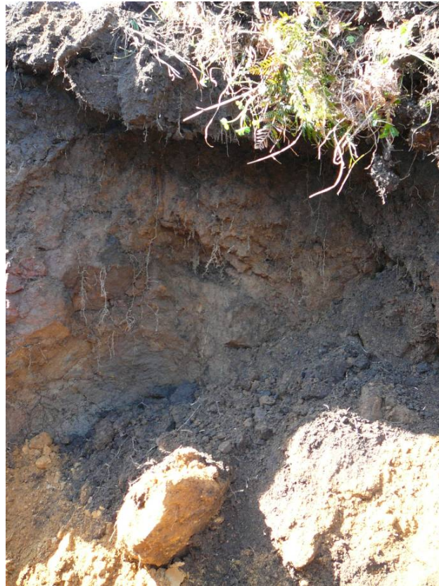
Photo 10: TP140 Note loosened rock mass in creep zone
