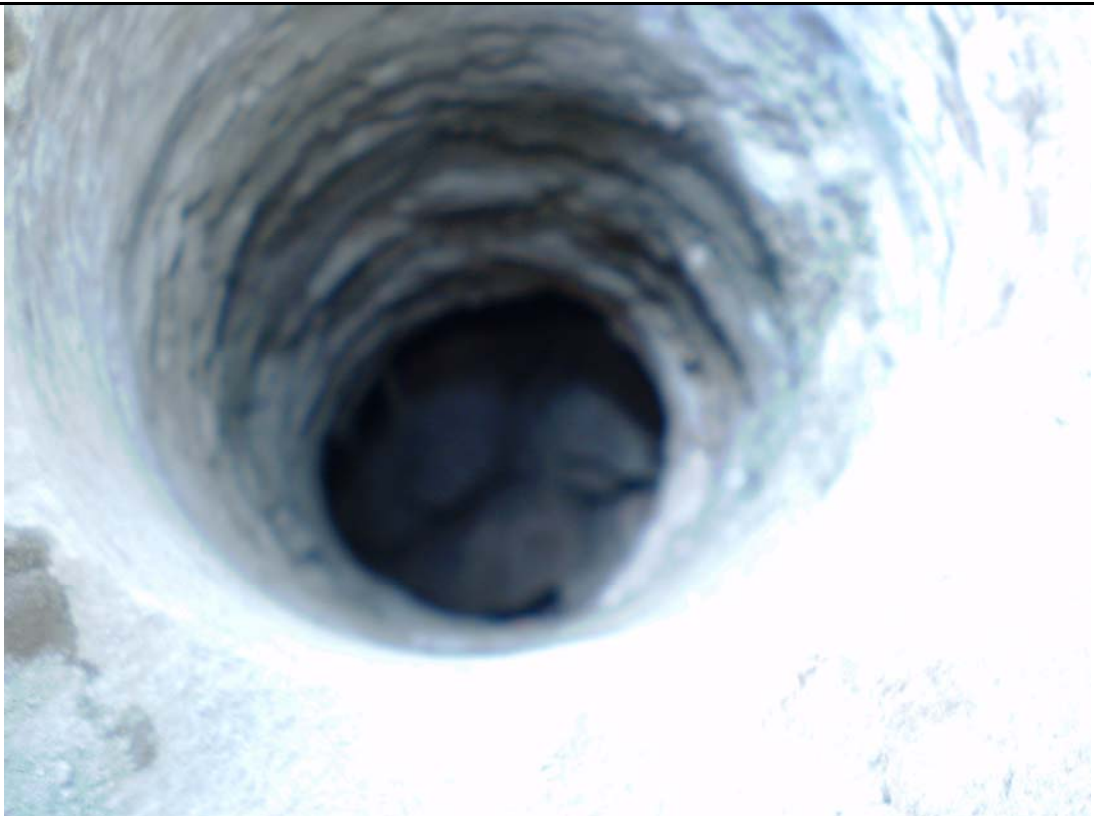
PHOTO 4: Conditions encountered in Bore 106. Large boulders were visible within a void at approximately 1.5 m bgl
