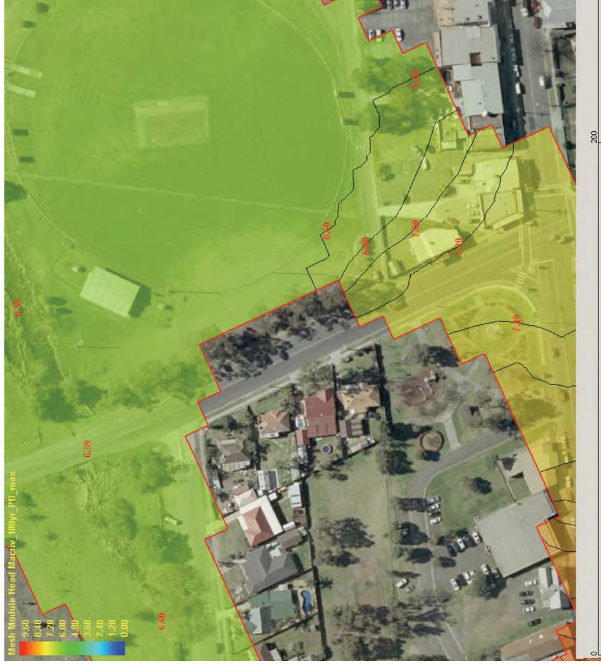
PMF Flood Levels - Tongarra Road
