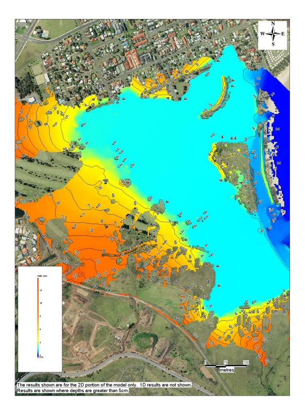
Figure 6.3 PMF Peak Water Level - Existing Scenario
