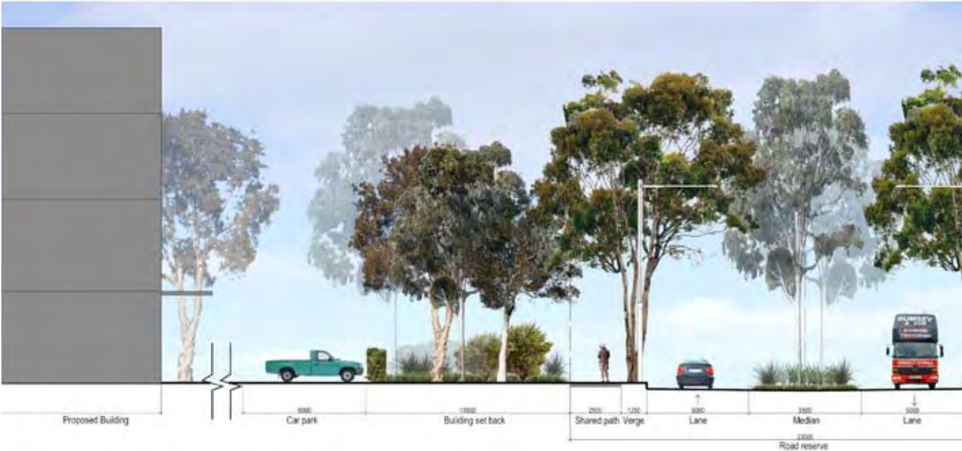
Section CC - 28m wide 'Private' Road Reserve (Collector road with 5m central median)
