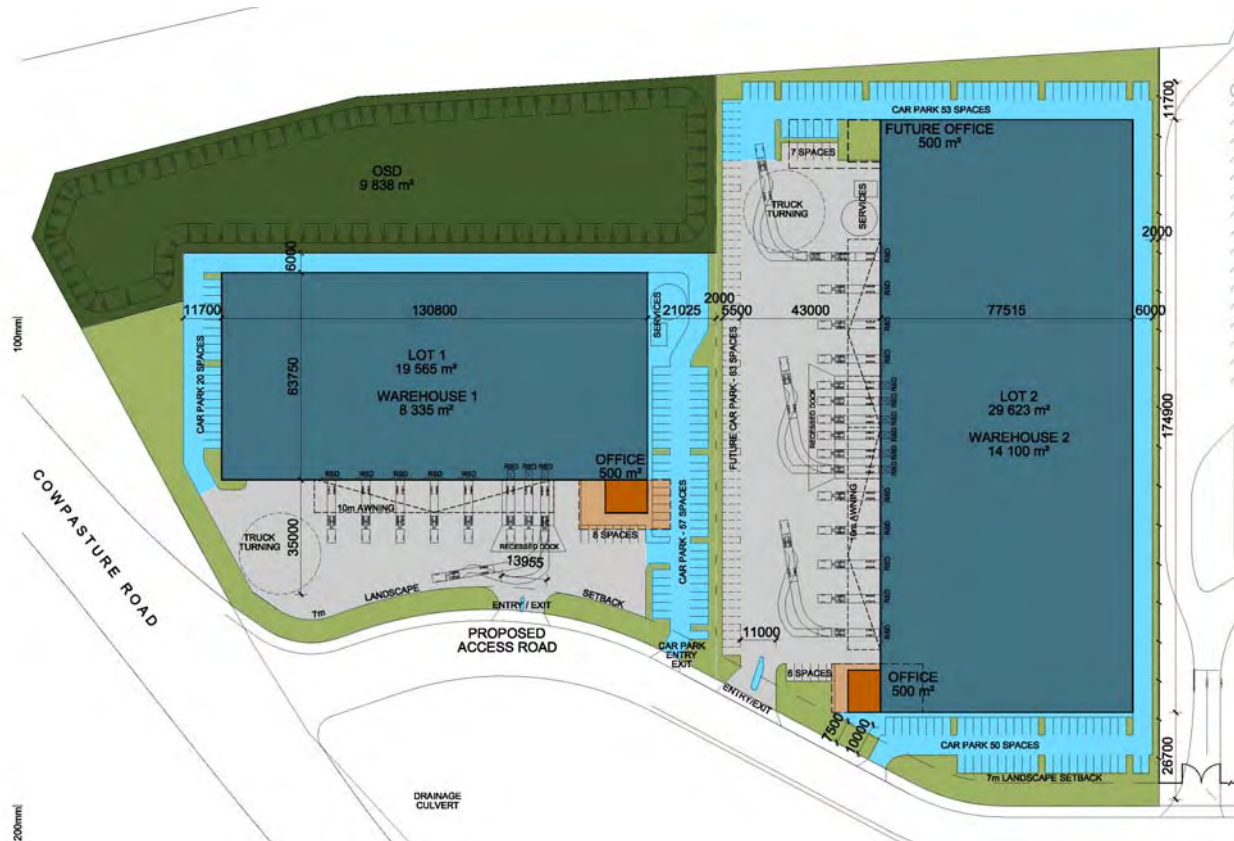
Figure 11 – Layout of warehouse / industrial buildings on the residual lot
